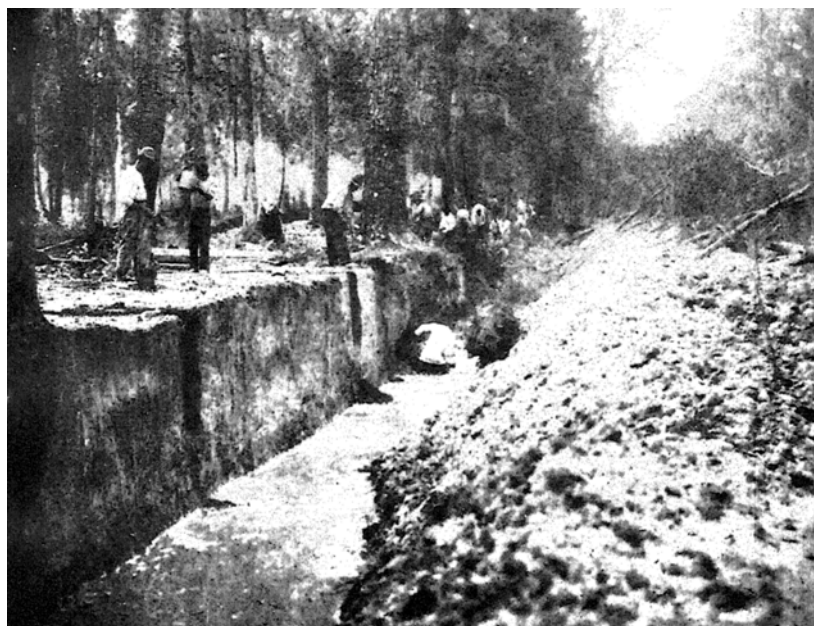
Figure 19. Phosphate mining. Top photograph shows ca. 1880 mining activity including 6x12 foot pits with phosphate rock thrown up in piles waiting to be moved to a tram by mule carts (courtesy of the South Caroliniana Library). Bottom photograph shows hand excavation of phosphate (from Waggaman 1913).
